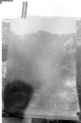
Molded fiberglass shim bolted to the bottom of the skeg lowers the aperture 10cm (4"). Note recess in bottom of shim for skeg bar. Original shaft hole filled and a new one drilled 5cm (2") below.
