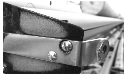
Without properly isolating these dissimilar metals, the stainless-steel fastener has corroded to the aluminum tang, making extraction very difficult.
