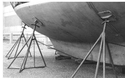
Sailboat properly tucked away: Boat rests squarely on keel blocks, stands balance the weight. Safety chains couple opposing jackstands to prevent sliding outboard under load.
