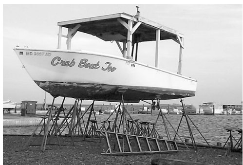
Sailboat jackstands raise this powerboat high and dry. Since stands are not designed to support a boat's weight, they may collapse, that's if strong winds haven't already launched the boat.
