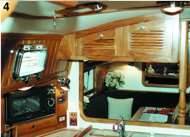
Galley Lighting: (1) Danish made Cabin multi-directional spotlight with 10-watt halogen bulb provides task lighting in the galley. To prevent shadows, mount the light in front of the work area. (2) Concentrated beam from a recessed downlight supplies task lighting only directly above the sink. (3) A fixture mounted behind a baffle sheds ample light to a galley countertop. (4) Practical illumination in the galley includes overhead general lighting, adjustable spot and under-coaming dome lights for task lighting.
