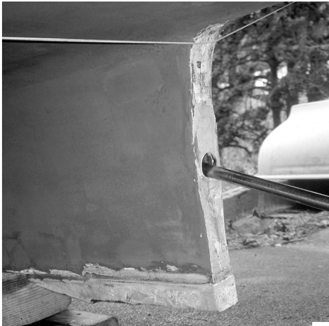
Molded fiberglass shim bolted to the bottom of the skeg lowers the aperture 10cm (4"). Note recess in bottom of shim for skeg bar. Original shaft hole filled and a new one drilled 5cm (2") below.
