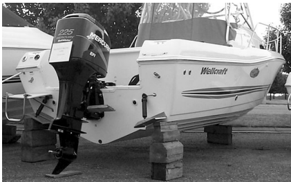
Without blocking under the keel to support the boat's weight, it's a shaky foundation destined for a topple.
