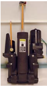
The oil reservoir on a late-model stern-drive trim pump. Oil level should be between the min and max marks with the trim rams fully retracted.
