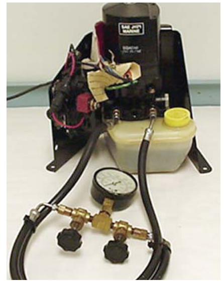
Your dealer can quickly check the condition of the pump using a test gauge.
