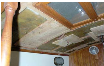
Removing all deck hardware involved removing fixed interior headliners to access thru-bolted deck fittings.
