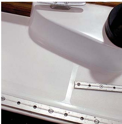
Completed painted deck shows smooth spillway breaking up the non-skid surface.
