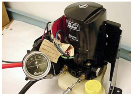
Checking the amperage draw with an inductive ammeter.
