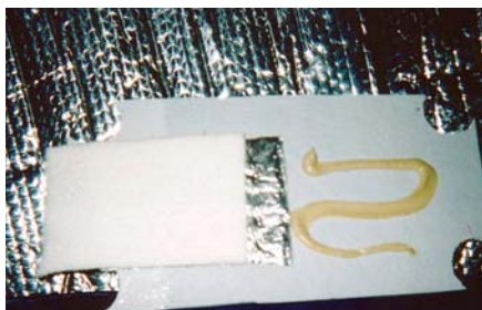
Test fiberglass board with Bull Dog Premium adhesive, Thermo-Foil and Fossfiber polyester marine liner.
