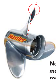
This prop has 0° flat rake as the face of the blade is perpendicular to the propeller hub and forms a straight line.
