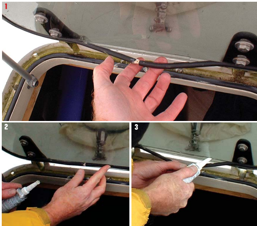
Steps to replace a gasket: 1 Loosen gasket on frameless hatch lid. 2 Press gasket back in place 3 Apply Sudbury Elastomeric sealant.
