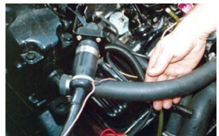
Soft or cracked hoses require replacement.
