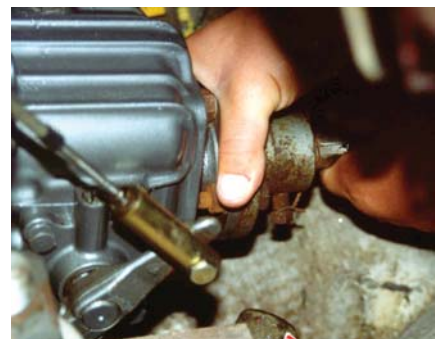
Testing the shaft coupler.
