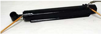
Check for oil leakage at seals and hose connections.
