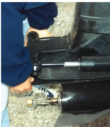
Sideways movement of the sterndrive more than 3mm (1/8") indicates wear to the steering arm linkage.
