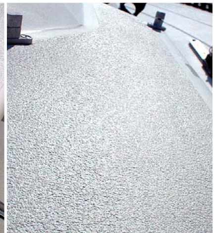
FIGURE 3 Example of stipple-style random non-skid on cabin top.
