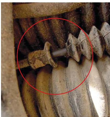
Damaged shift bellows can sink a boat.
