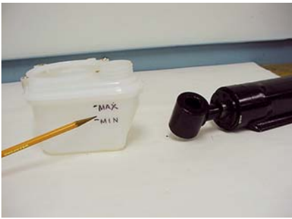
The oil reservoir on a late-model stern-drive trim pump. Oil level should be between the min and max marks with the trim rams fully retracted.
