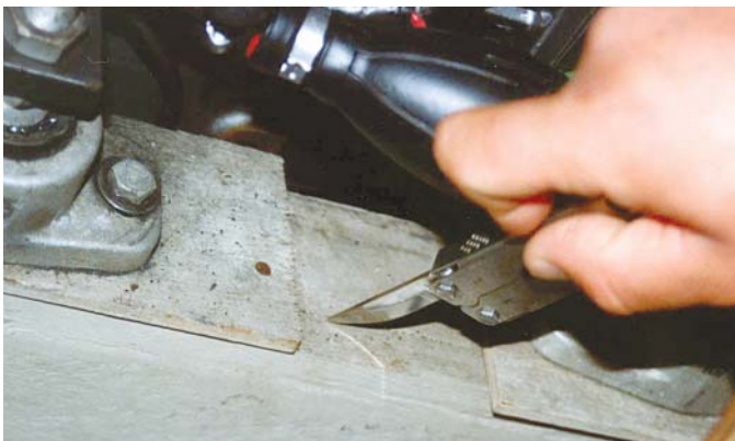
Inspect the condition of the engine stringers and engine mounts for movement.
