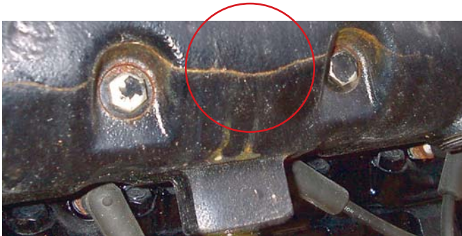
A cracked manifold.
