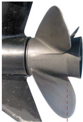
This prop has 0° flat rake as the face of the blade is perpendicular to the propeller hub and forms a straight line.
