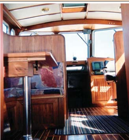
Ceiling in main cabin is foam-backed vinyl on 3mm (1/8") marine plywood with mahogany battens.
