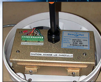
(top) Sea Tel model 1898 is designed for power and sailboats as small as 30' (9.1m). (bottom) Interior of 3918 Sea Tel antenna.
