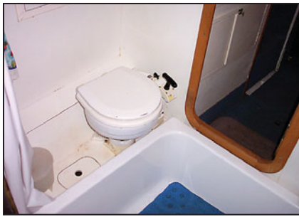
This shows the area where the existing marine head was located. It is set down into a depression by the bath tub/floor combination.
