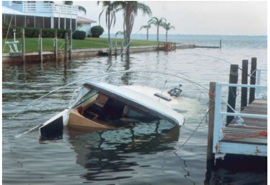
Surprisingly, I/Os with leaking bellows accounted for 44% of sinkings at the dock.
