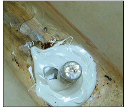
Adding sealant on the inside of a keel bolt may not always work.
