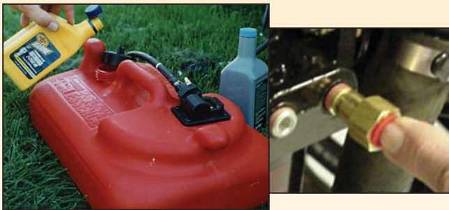
Outboard tank containing "storage soup" connects to fuel inlet on engine.
