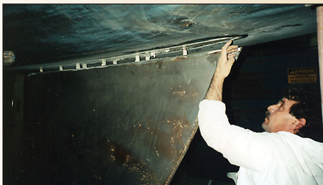
Fin keel dropped ready for new sealant and chocking epoxy.
