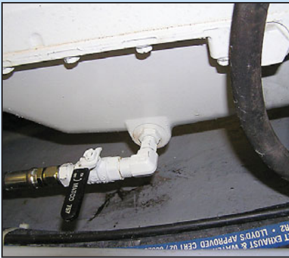
A dry bilge that persists beneath the engine verifies no leaks.
