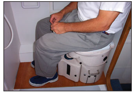
This photo shows the space required to comfortably use the head. Length from rear bulkhead to the bulkhead in front of the author's feet is 36" (91cm). Width of the platform is 14" (36cm). Air Head itself measures 19" deep x 16" wide x 19.5" high (48cm x 41cm x 50cm).
