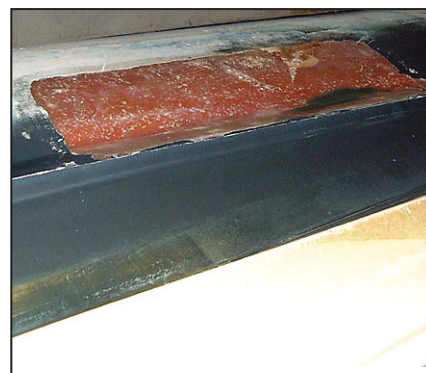
Repairing a delaminated area on the hull of a lifeguard rescue skiff.
