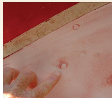
Wet core below the waterline means major repairs.
