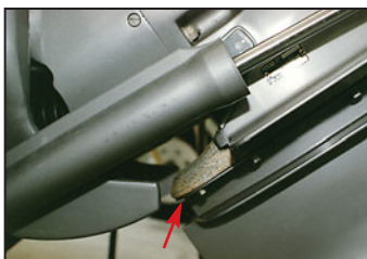
Drive anodes come in various shapes. Carry exact replacements for your engine.
