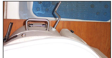
This photo shows the space required to comfortably use the head. Length from rear bulkhead to the bulkhead in front of the author's feet is 36" (91cm). Width of the platform is 14" (36cm). Air Head itself measures 19" deep x 16" wide x 19.5" high (48cm x 41cm x 50cm).
