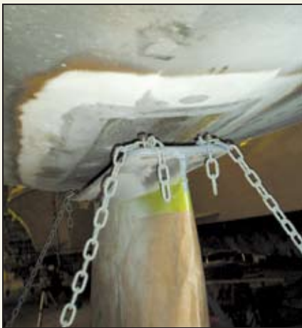
The easiest way to handle a T-Bird keel is leave it upright on the trailer, securely restrained.
