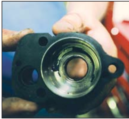
(left) Water pump housing. (right) Damaged water pump body shows signs of scoring caused by overheating.
