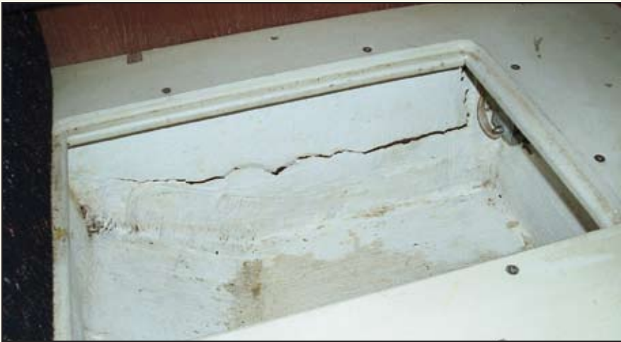
(top) The popped secondary bond at the bottom of a main bulkhead is not a good sign. (bottom) Note the crack in this keel sump near the forward keel bolt.
