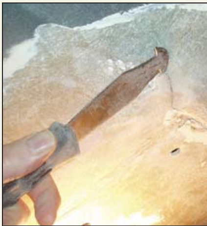
Cracks from old grounding incidents, never properly repaired, weakened this hull.
