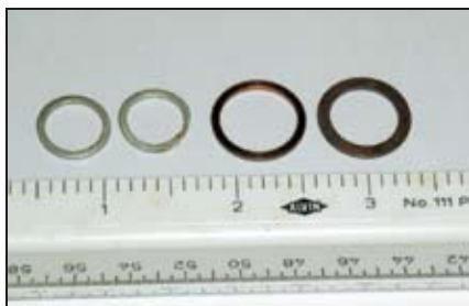
Corroded and bent metal crush washers shown on the left; new ones on the right.
