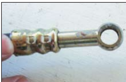
Banjo bolt fitting on a fuel line.
