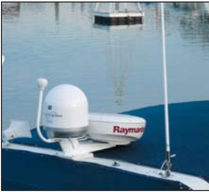
Grouping antennas can create interference with certain electronics.
