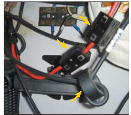
Doughnut-shaped and clip-on type ferrites prevent radio frequency interference. If possible, make a cable loop or two through the ferrite.
