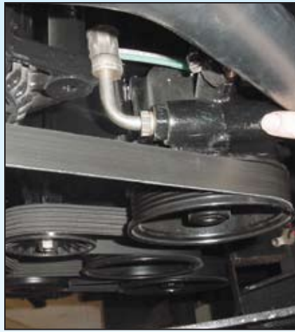
Typical power steering belt system.
