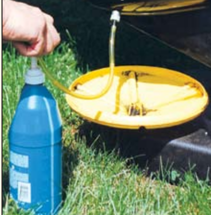
(left) Drain/fill screw at the base of the lower unit housing. (right) Vent screw located on the upper gear housing.
