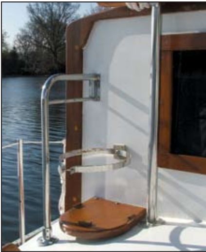
Tank platform, strapping and protective handhold.
