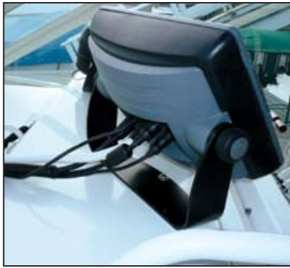
When routing the cabling be sure to leave extra length to allow for easy turnaround or removal of the display.
