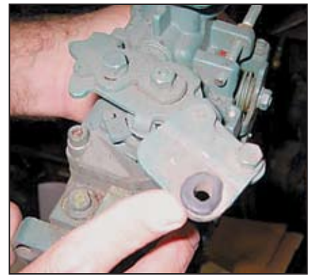
Worn bushing on a fuel injection pump where a clevis or pin post throttle fitting might go.
