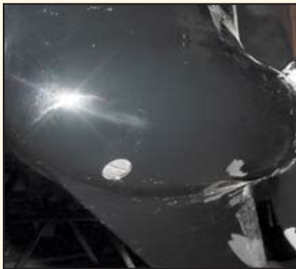
(left) Drain/fill screw at the base of the lower unit housing. (right) Vent screw located on the upper gear housing.
