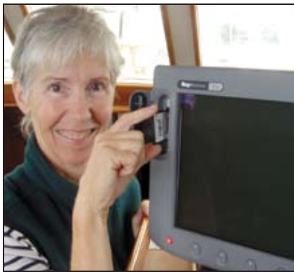
Author's wife inserts chart card into slot on chartplotter. Electronic charts provide more information than paper charts and are read by most chartplotters.
