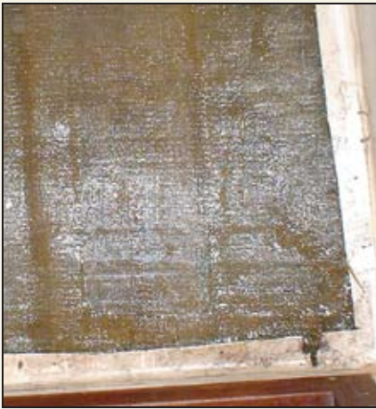
Fresh new laminate of 1810 Stitchmat. Note the color difference from the delaminated stuff, visible in the "before" photos.
