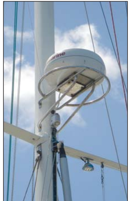
All of the new radar products can be owner installed, as there are no calibration or alignment requirements requiring a licensed electronics' technician.
