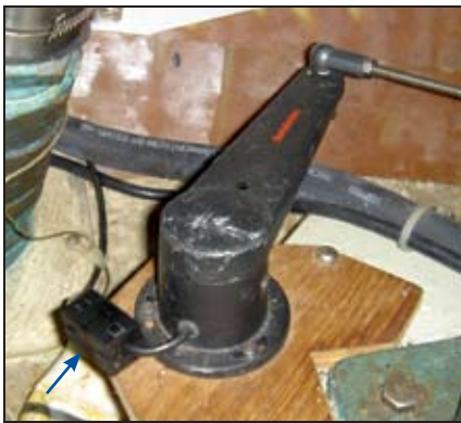
Rudder position transducer mounted with ferrite on the cable.
