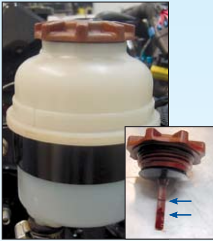
Maintain the power steering fluid level at the correct levels on the dipstick.
