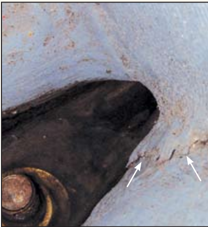
(top) The popped secondary bond at the bottom of a main bulkhead is not a good sign. (bottom) Note the crack in this keel sump near the forward keel bolt.
