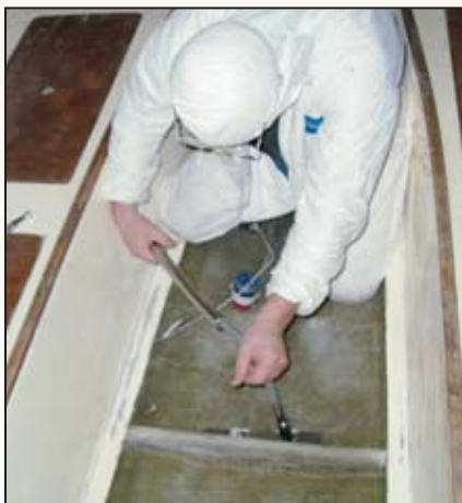
Tightening the keel bolts using the 40-years experience torque gauge. Don't do this on your boat — always use a torque wrench.
