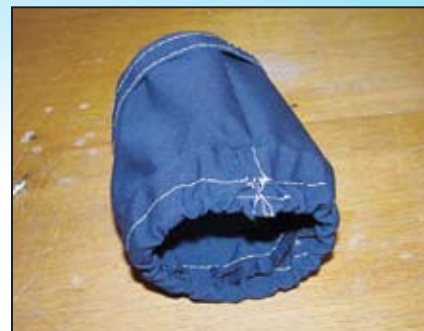
9 Shock cord crossover sewing detail.
