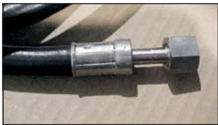
Examples of compression fittings: (top) Assembled bronze compression fitting with plastic hose. (bottom) Swaged steering hose fitting.
