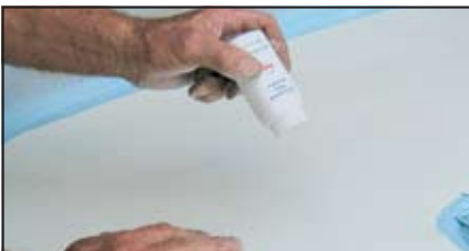
To minimize squeegee friction a dusting of talcum is recommended.
