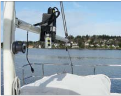
(left) New saddle attaches boom gooseneck to the mast and electric winch mounts to inboard end of the boom. (middle) Custom cover weatherproofs the winch.
