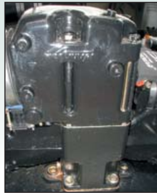
In boats where the waterline is higher, the exhaust elbow is raised to gain a safe height above the waterline. This photo shows a 6" (15cm) exhaust riser mounted between the engine's exhaust manifold and the exhaust elbow to compensate for waterline height problems. The waterline can change drastically due to loading and sea conditions and exhaust system installation must account for these conditions.
