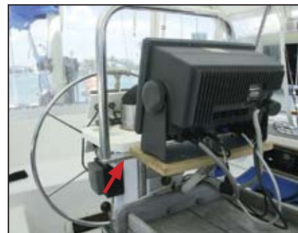
Figure 4 (top) New rigid and strong grab rail offers a clear view of the screen. (bottom) Back side of the plotter shows additional construction details.
