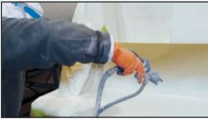
The subsurface must be a consistent matching gelcoat so a sprayed prime coat is mandatory on large repairs.
