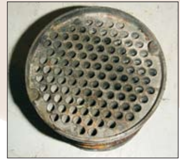
(left) Typical tube bundles. (right) End view of a tube bundle shows the small 1/4" (6mm) diameter tubes.
