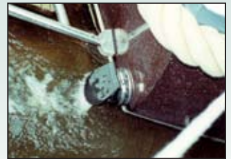
Vetus transom exhaust flapper with thru-hull connects directly to the exhaust hose.
