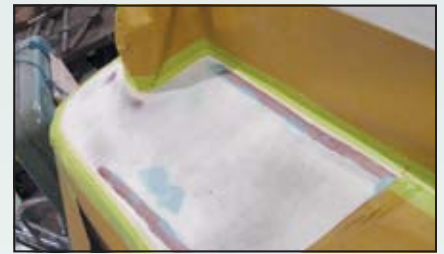
Careful masking defines the edge of the new non-skid pattern.
