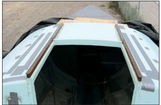
Arrived safely and it's time to remove strips of tape covering holes drilled to dry out the deck core. We were lucky that the truck did not encounter rain en route.
