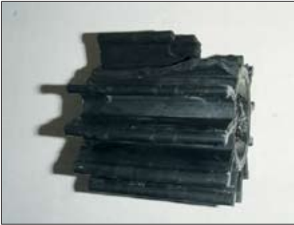
Seawater impellers with missing blades that are now likely resting in the heat exchanger tube bundle.
