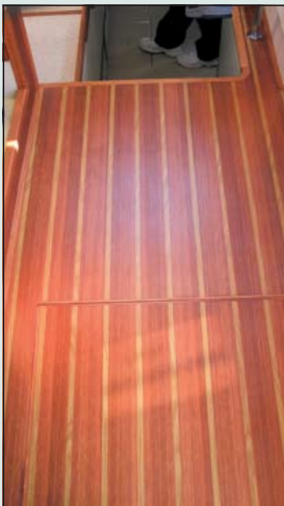
Island Packet's new PY Cruiser uses a renewable alternative to oak, cherry and mahogany known as Lyptus, a hybrid hardwood made from Eucalyptus trees, grown on plantations in Brazil and that reach harvest size in just 15 years.
