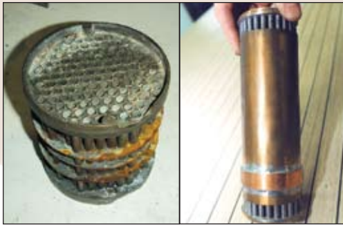
(left) Typical tube bundles. (right) End view of a tube bundle shows the small 1/4" (6mm) diameter tubes.
