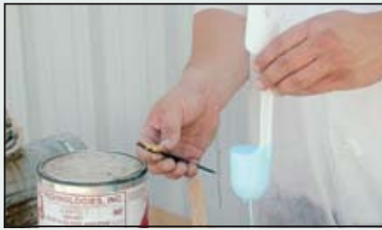
Thin the gelcoat. It should take 45 to 50 seconds to run through a #2 Zahn cup.
