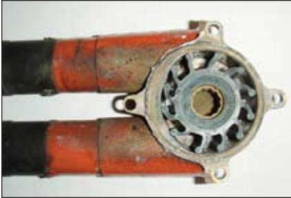
(top) Seawater pump with a corroded plate and fasteners that need replacing. (bottom) Impeller positioned in a seawater pump.
