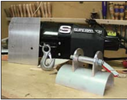
Restored winch and mast saddle components.
