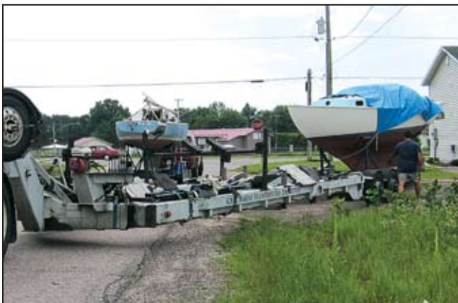
With the cradle turned and on blocks, the boat was finally ready for loading onto the trailer.
