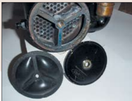
Heat exchanger end shows tubes, cover and gasket. Covers crack if overtightened.
