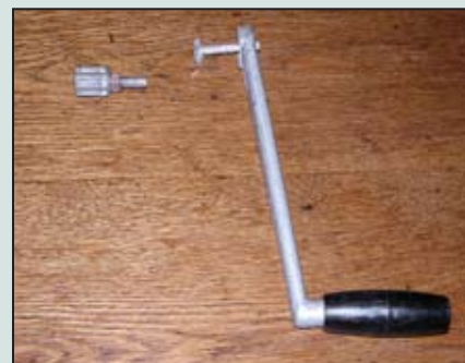
Custom-made adapter lets you power winch with a right angle drill.
