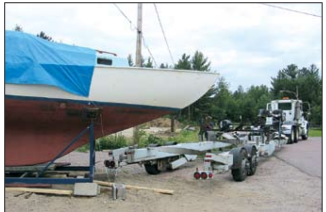
Grey hairs, anyone? The truck slowly drags the cradle forward onto blocks to allow 8" (20cm) minimum clearance for the hydraulic lift. Since the truck was too long to back straight into the driveway, the cradle was also dragged to one side to allow access.
