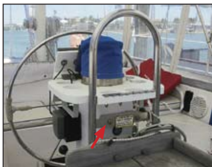
Figure 2 Details of original rail (plotter removed) that is bolted to the cockpit sole. Note placement of support brace.
