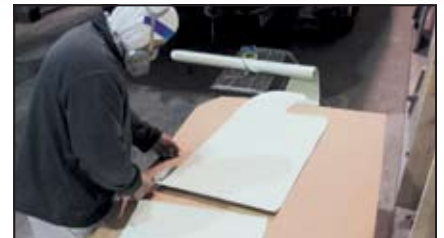
The Flex-Mold is easily cut to a pattern.
