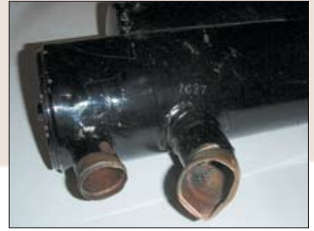
Heat exchanger with a bent outlet due to overtightening a hose clamp.
