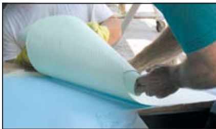
Doing the wave: push the gelcoat ahead when laying down the Flex-Mold.
