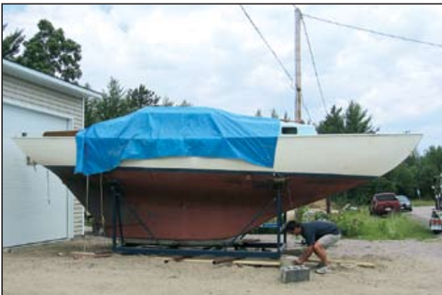
When we arrived, the cradle was resting on 4" steel pipes that the seller had used to roll it out of the garage. Here boat hauler Dave Kopriva positions cement blocks under the cradle.
