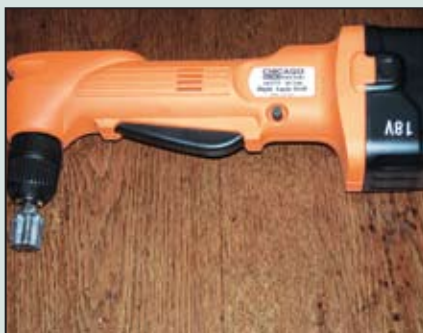
Custom-made adapter lets you power winch with a right angle drill.
