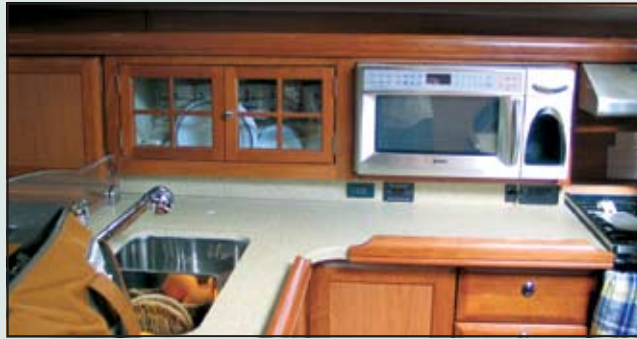
Interior cabinetry and cabin soles in the newest offering from Hunter Marine are made of maintenance-free, scratch and scuff resistant veneer over plywood with an aluminum oxide finish. No need for oil or varnish in this interior.
