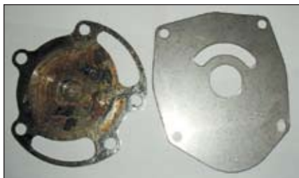
Replace worn impeller wear plates when servicing a seawater pump.
