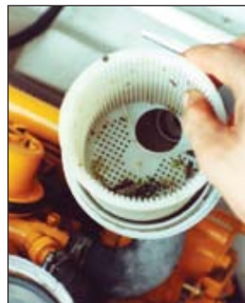
(left) The seawater strainer filters debris, sand, weeds, etc. before they get into the engine. (right) All strainers have a removable filter or screen that should be inspected and cleaned before every engine startup.
