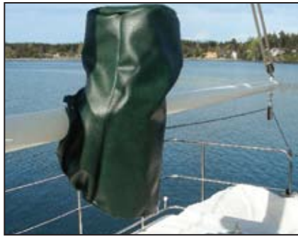
(left) New saddle attaches boom gooseneck to the mast and electric winch mounts to inboard end of the boom. (middle) Custom cover weatherproofs the winch.
