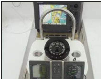
Figure 1 The pedestal-mounted grab rail obscures the plotter screen.
