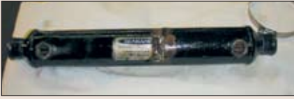
Replace expendable oil or transmission cooler when corrosion is noted at soldered joints.
