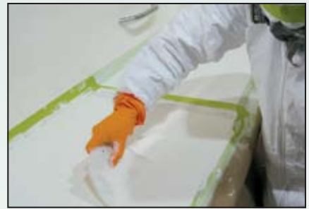
Squeegee out excess gelcoat in all directions until the Flex-Mold lays flat and even.
