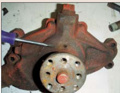
Weep port of a seawater circulation pump has been leaking for some time. Replace this type of pump as rebuilding is not practical.
