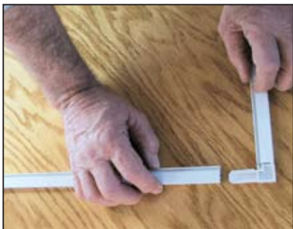
Push side strips onto corner pieces.
