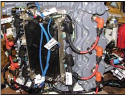
Computer and ignition module installed.
