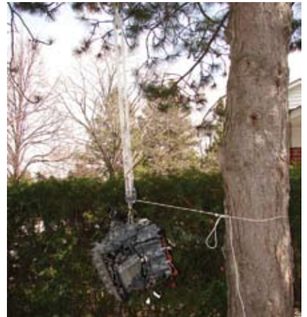
Power head tied off to the tree, while boat is moved out of the way.
