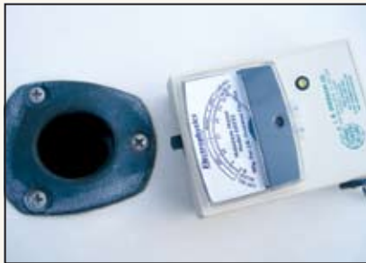
(left) Warning sign: A moisture meter can help confirm that the brown ooze seeping from a fiberglass laminate (right) indicates a wet, rotten core.
