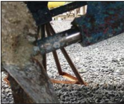
The evidence of extreme shaft movement, caused by broken engine mounts, is seen in the polished areas of the shaft. It's amazing that the owner didn't notice or the shaft did not break.
