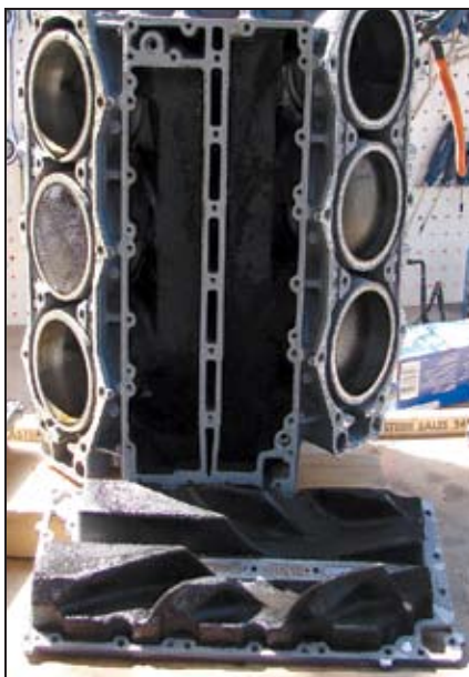
Exhaust plate cover removed. This is the carbon and oil build up from the last rebuild just one year before. I removed all the rough areas in the sand-cast block with a small die grinder to allow for better exhaust flow.
