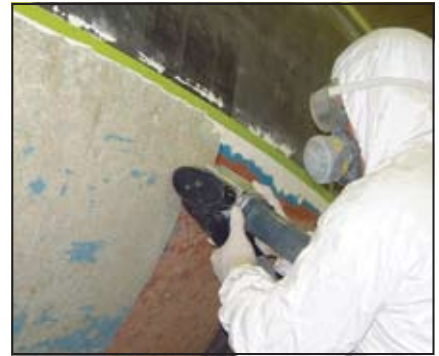
More severe osmosis requires complete removal of the gelcoat and sometimes part of the laminate using a peeler.
