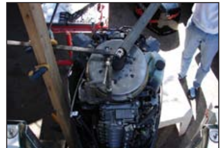
Breaker bar as shown from above. This set up worked fine.
