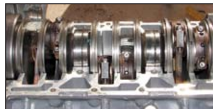
Shown are the six connecting rods attached to the crankshaft, two bearing raceways and locating wire and the nine crankshaft seals. Be careful when removing the crankshaft as I broke one of the seals and decided it was prudent to replace them all.
