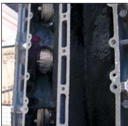
View of the scored number four piston through the exhaust port.
