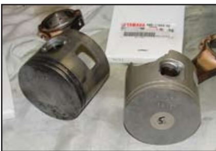
Old piston beside new piston. No rings installed. Only the piston was replaced. The rod, pins and bearings were in very good shape and only required cleaning and lubing. New C clips were used on all pistons as they had been removed from the rods for checking and cleaning.
