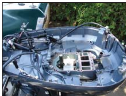
Base and lower unit cleaned and ready for the power head. When cleaning off the old gasket material block all openings to ensure no debris gets in. New gasket in place.
