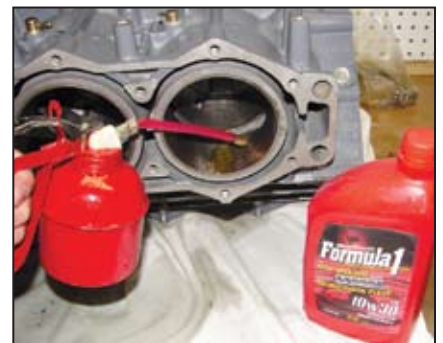
The machine shop recommended using 10X30 oil to lubricate cylinders prior to installing connecting rod bearings and pistons.
