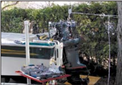
Wire rope and shackle are wrapped around a tree branch and a rope pulley attaches to the powerhead to lift the powerhead off the lower unit.
