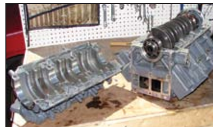
The two half's of the crankcase are separated. The crankshaft is now exposed.
