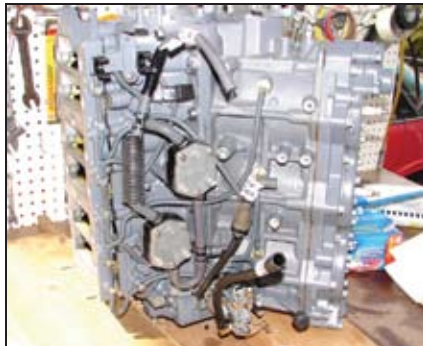
Port side of the engine. This view shows the two fuel pumps and the oil pump located on the bottom.
