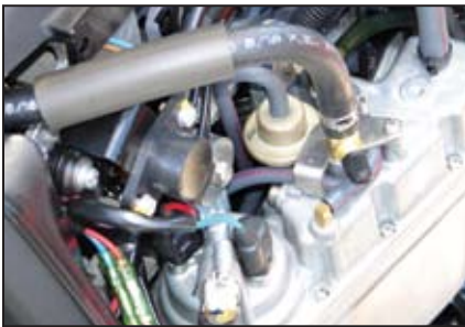
Fuel injection pump from the top. Showing Schrader valve and pressure regulator valve.
