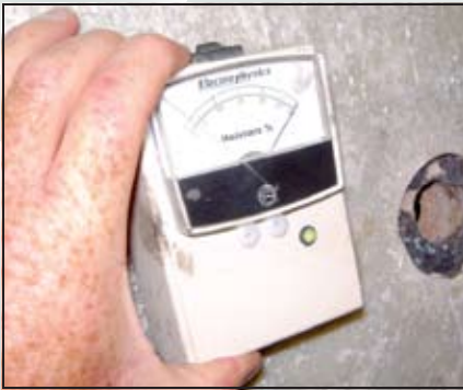
Moisture meter shows that this hull is affected by moisture.
