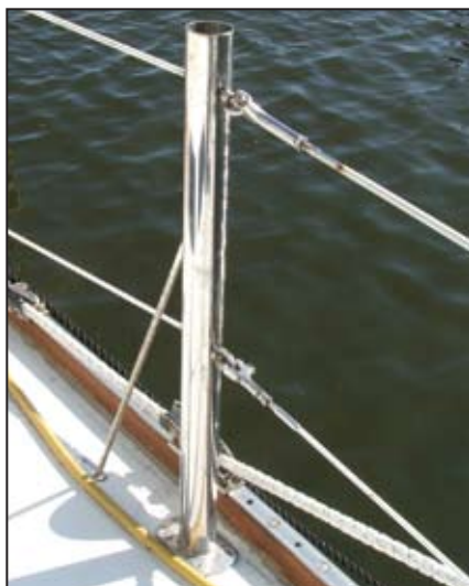
New stanchion/stovepipe installed on deck.
