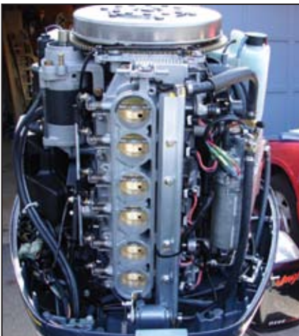
Intake showing air intake and fuel rail for injectors.
