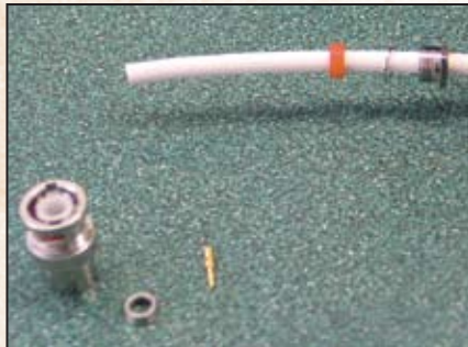
Components of a BNC connector for coaxial cable.
