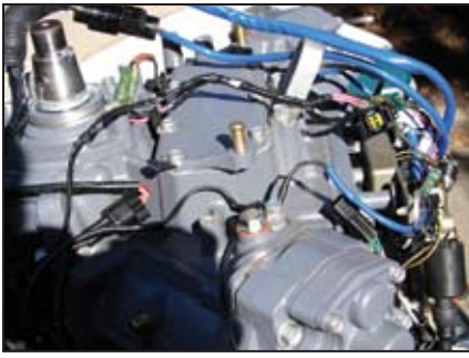
Picture of the ground wire running to the top of the port head.
