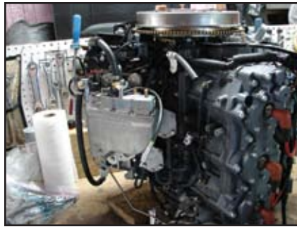
Install the fuel pumps before installing the high pressure fuel pump. It makes it easier.
