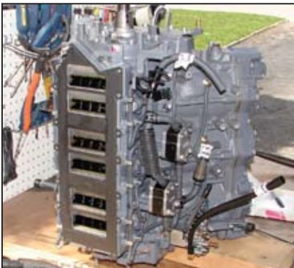
View of the intake without the intake assembly. The six rectangular openings on the second intake plate are for the reed valves.
