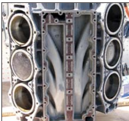
The exhaust cover removed exposes the water jacket section. I had deburred this area to allow good water flow on the first rebuild and touched up the finish with some extreme high heat paint (shown in red) rated at 1,400F (760C) but it didn't survive well on the starboard side. I lightly sanded this area to prevent paint flecks gumming up the cooling system.
