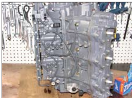
Port side of engine. Bleed hoses attached to reed plate on the left side. The silver section at the bottom is the area that the oil pump bolts on to. The pump is driven by a gear that runs off of the crankshaft.
