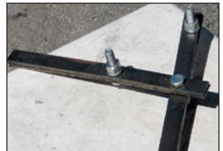
Home-made flywheel wrench (breaker bar) made of 1/4" by 1" (6mm by 25mm) flat bar has two pieces bolted together to fashion a strong handle and then two pieces of flat bar, 10" (254mm) long, bolt to the handle about 6" (152mm) from one end to create a pivot. A minimum 1/2" (12mm) hole is drilled about 2" (50mm) from the handle end, past the pivot point and opposite to the pivot connection bolt.
