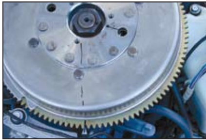
Flywheel and hold down nut. This must be torqued as specified in the service manual.
