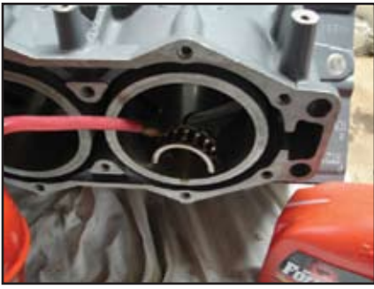
Lube connecting rod bearings.
