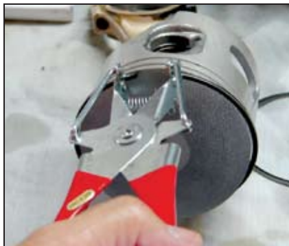
Installing new piston rings on new pistons using a spreader. Be sure the ring is installed the right way up. Also make sure the notch in the ring goes around the pin in the groove when clamping with the piston ring compressor. Some times a little twist of the piston will set it right.
