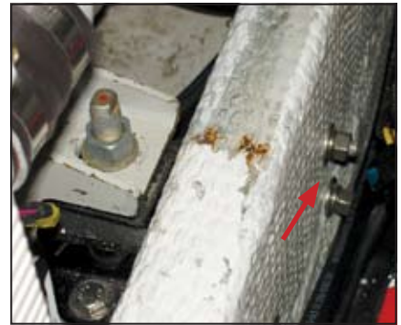
(left) Poor installation: there's no space to adjust the engine height on this mount. (right) Ideal positioning of the engine bracket on the mount allows for height adjustment as the mount loses stiffness with age. Cross bolts for mounting brackets are loose (shown by arrow) and the stringer likely decayed. Nuts must be tight without crushing the stringer.
