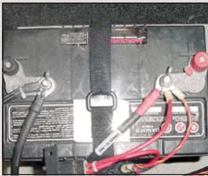
(left) New motor rigged with wing nuts holding on the battery cables. (right) Wing nuts replaced with locking nuts tightened with a torque wrench.
