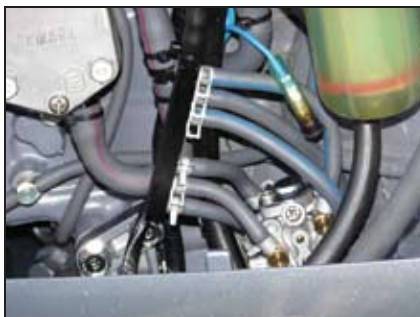
Oil pump and hoses
