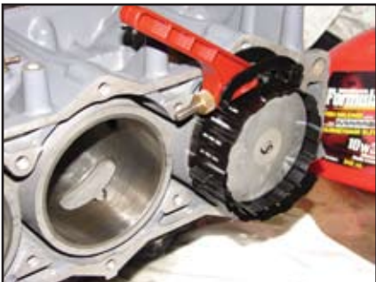
Piston being installed.
