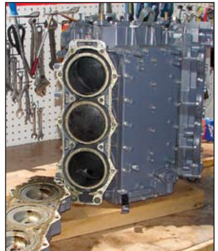
Port head removed. Bolts are bagged and tagged. Notice the lack of carbon build up as compared to the first rebuild (shown on page 58) for a timeline that is less than one year.
