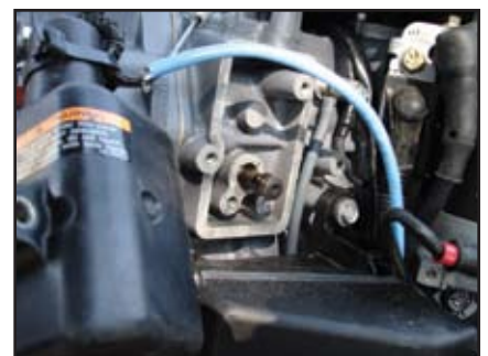
After the initial break in, the oxygen sensor joint is removed. Oil build up is from assembly oil, standard engine oil and oil in the tank for engine break in. Because the break in does not allow for high rev's for the first part I used the old oxygen sensor for this part. This also allowed me to test it as per the new testing method. It failed.
