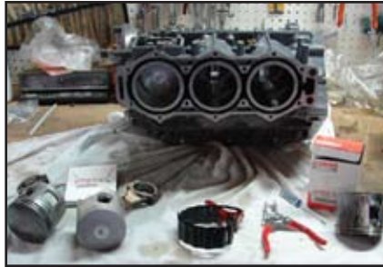
Ready to install new pistons.
