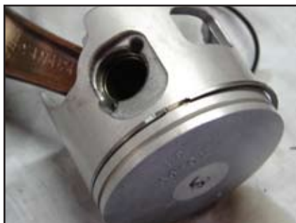
New piston ring installed. Make sure the ring is installed the right way up. Also make sure notch in the ring goes around the pin in the groove when clamping with the piston ring compressor. Sometimes a little twist of the piston will set it right.
