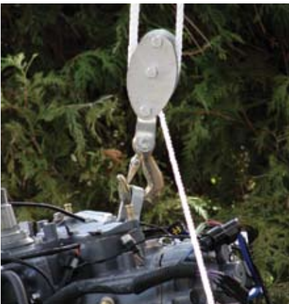
Rope pulley attached to the top of the engine.
