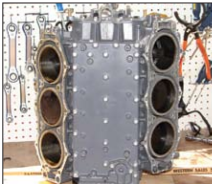
Looking at the back of the engine. This is the exhaust port cover. It was under the computer and ignition coils. Both heads are now removed.
