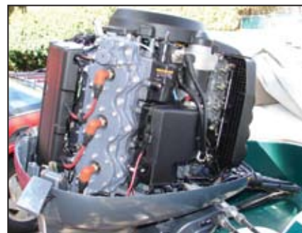
Starboard side of engine showing, starter, oxygen sensor, fuse box and shifter connections.
