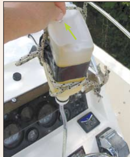
Purging the air from this '90s vintage SeaStar side mount hydraulic steering was long overdue.
