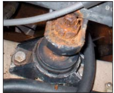
Rusted nut makes it impossible to adjust bracket height.
