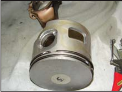
New rings and piston oiled.
