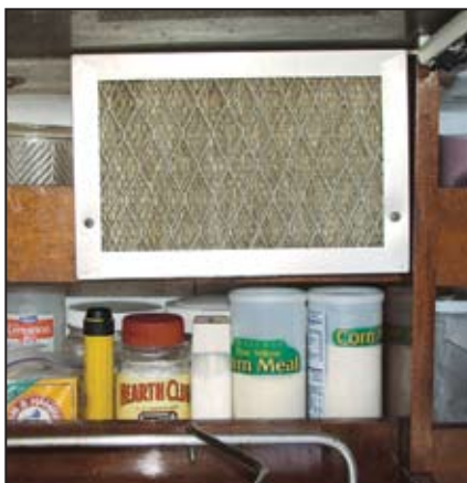
Metal filter installed in front of blower locker.
