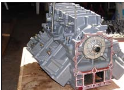
View of the bottom of the block. The two exhaust ports can be seen at the bottom. The round section is the lower crankshaft cover. You must mark the orientation of this cover. It also shows the crankcase bolts being removed.
