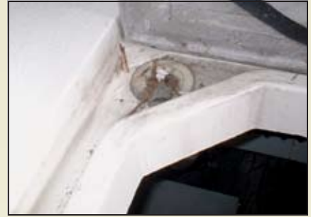
Cockpit drain plugged with debris caused water to flow over the hatch flange and flood the engine compartment. The condition went unnoticed for six months of dry storage.
