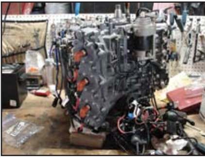
Starter and the computer and ignition coil module installed. Starting to wire the fuse box.
