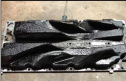
Inside of exhaust port plate. Prior to cleaning. Not easy to clean!!
