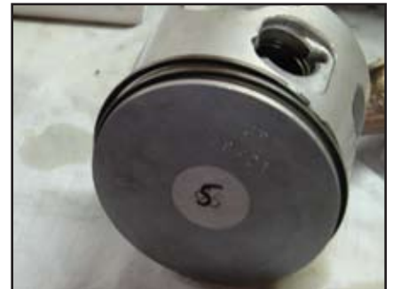
New rings on new piston.
