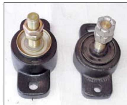
An example of two very similar mounts with differently sized fastener mounting bolt holes.
