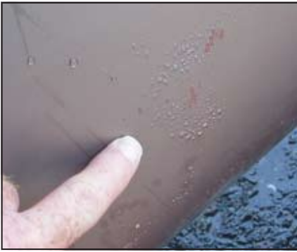
A rash of blisters, limited to the antifouling, is a very minor repair.
