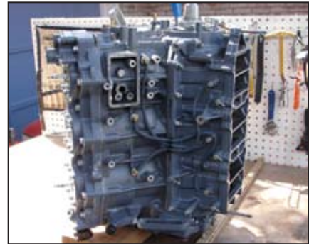
Starboard side of engine. This picture was taken for the bleed hose layout. The engine is now down to the heads on the left and the crankcase. It is split in the middle around the crankshaft. The rectangular section and the oily back hole is where the oxygen sensor sits.
