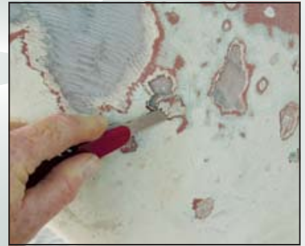
Blister analysis requires a sample for examination. A penknife or chisel cuts around the perimeter of the keel blister and peels it back.
