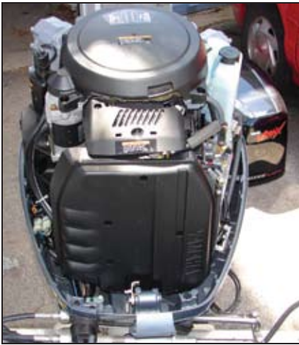
Air intake Silencer and flywheel cover. This covers the air intakes and fuel injectors.
