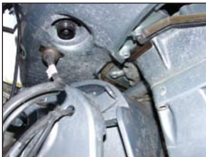
Removing hidden power head bolts.
