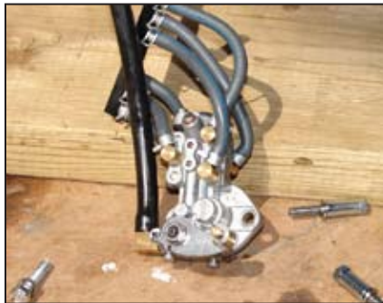
Oil pump and screws. The oil control rod attaches to the pivoting section where the cotter pin is located.
