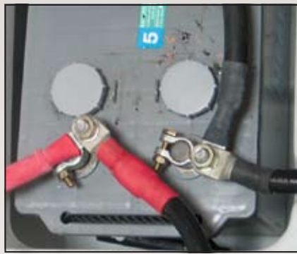
(left) New motor rigged with wing nuts holding on the battery cables. (right) Wing nuts replaced with locking nuts tightened with a torque wrench.
