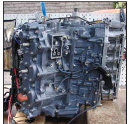
Powerhead is lowered and braced on the workbench. Fuse box is removed from starboard side and is sitting behind the engine.
