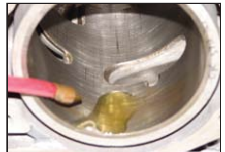
Lube cylinders prior to installing pistons. Wash and dry the block after getting it back from the machine shop to remove all dirt and metal fillings. I washed mine twice and used a pressure sprayer to blow it out then dried it by hand and oiled it down to prevent rusting. Then covered it with a clean sheet to keep the dirt out.
