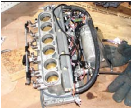
Intake assembly, including high pressure fuel pump and float bowl, butterfly air intake valves, fuel rail and injectors.
