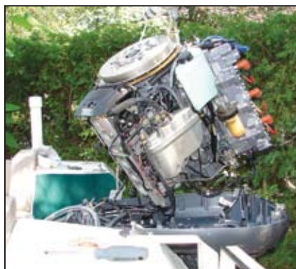
Lowering the powerhead in place requires three people: one to lower and two to situate.
