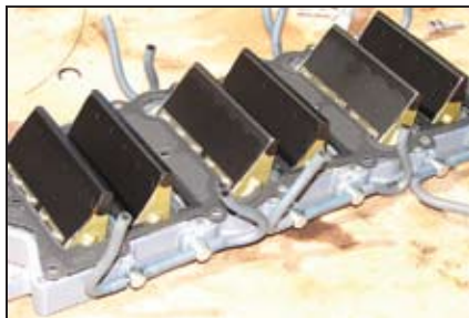
This is the reed plate. Replaced reed valves are carbon fiber and react better than the original steel reeds.
