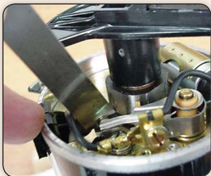
Setting point gap with a feeler gauge.
