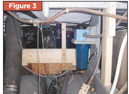
Typical temporary cabin sole support.
