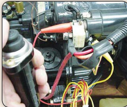
Remote starter switch connected to starter solenoid.
