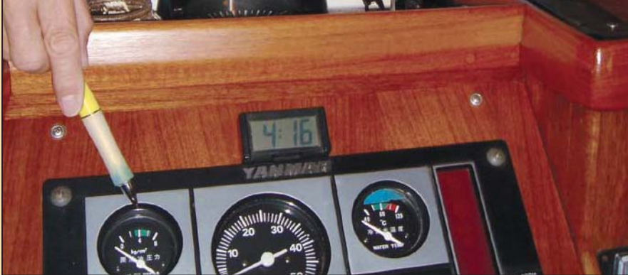
Author points to the faulty oil pressure gauge.
