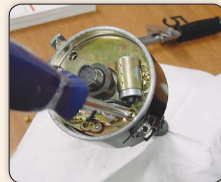
Removing the breaker plate.
