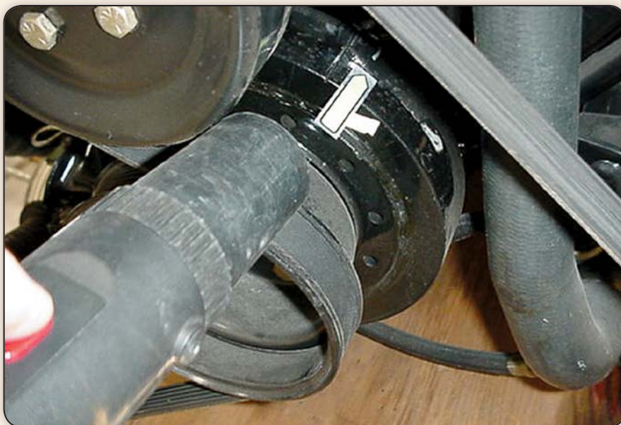
Checking base timing with a timing light.
