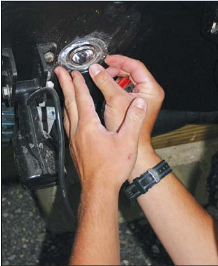
Set the lines in the lens to vertical when installing.
