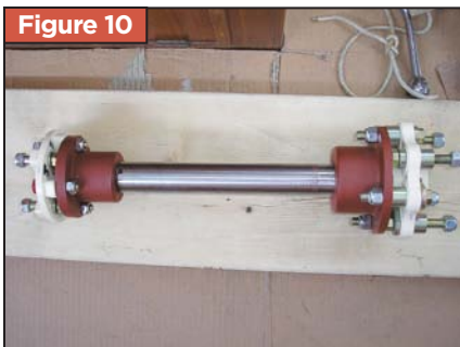
New shaft extension with R&D flexible couplings installed.
