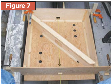
Template for locating the new engine mounting brackets.
