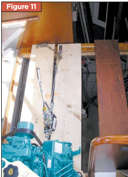
Template for locating the new engine mounting brackets.
