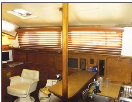
Before: Teak plywood damaged by 28 years of the inevitable water leaks around the portlights.
