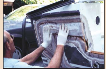
Fiberglass tape is laid over the sections where the fiberglass laminates butt together, saturated with epoxy, and then rolled to remove air bubbles.
