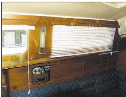
Before: Teak plywood damaged by 28 years of the inevitable water leaks around the portlights.
