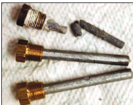
Check the heat exchanger and any zincs. If not maintained, there may be expensive corrosion repairs.
