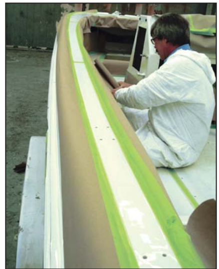
Masking for non-skid application on two classics: (top) Hatteras 53, (bottom) Boston Whaler Outrage 21.
