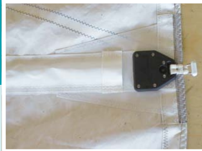
(top) Double fabric construction at the luff consists of the batten pocket sewn over a glued-on triangular protective patch. (bottom) Finished luff with batten end cap that solves chafe and compression loading troubles at the luff.
