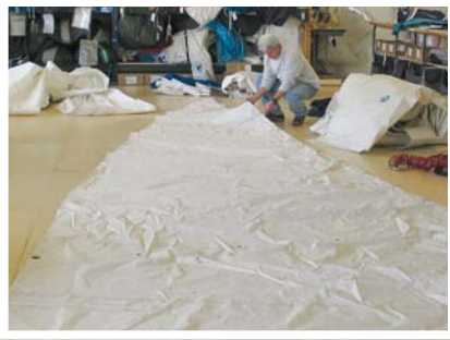
Initial inspection by a sailmaker qualifies the sail for a full-batten conversion.
