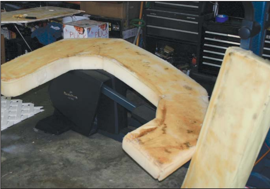
Mildewed foam is treated with a bleach solution followed by denatured alcohol.
