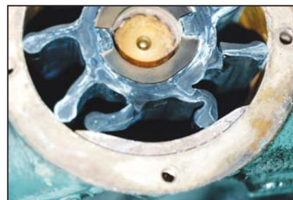
(top) Remove the water pump cover and (bottom) check the raw-water pump impeller for damage.
