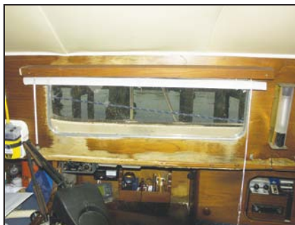
Before: Teak plywood damaged by 28 years of the inevitable water leaks around the portlights.
