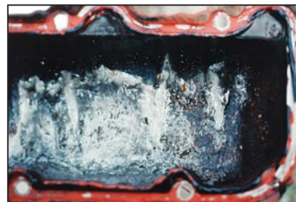
Emulsified (water contaminated) oil in the valve cover.
