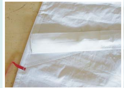
“Flip-flop” pocket for cruising sails compresses the batten and “seals” the batten end so it cannot open should it strike a backstay or topping lift.
