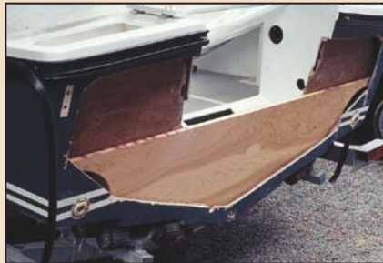
Fiberglass tape is laid over the sections where the fiberglass laminates butt together, saturated with epoxy, and then rolled to remove air bubbles.
