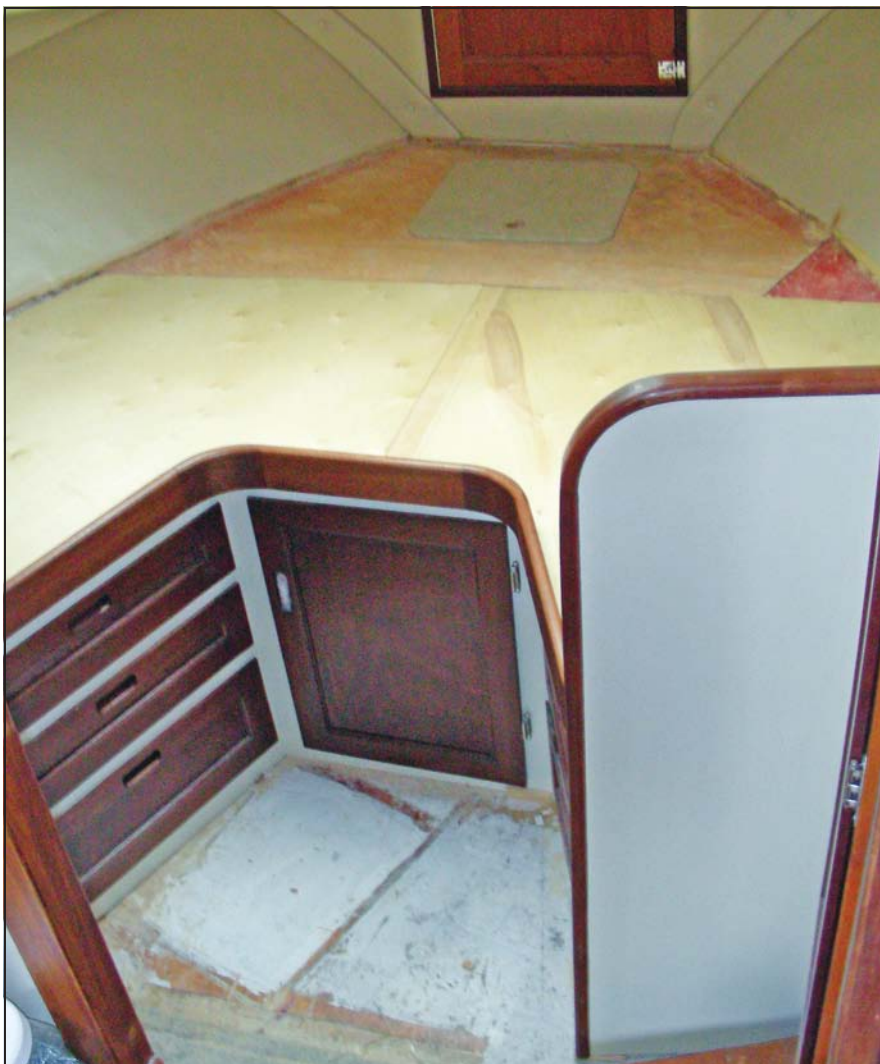
Deck of 3/4" (19mm) plywood screwed in place. This is covered by a felted fabric-on-rubber overlay.
