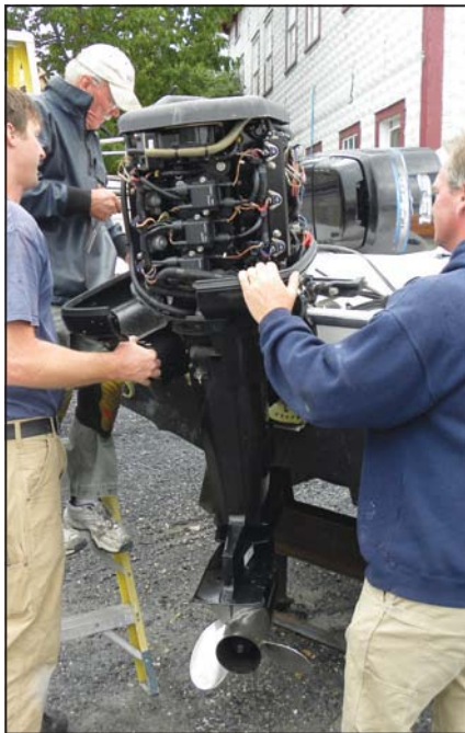
"Fog" carbureted engines by spraying engine storage seal into the carb.
