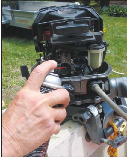
"Fog" carbureted engines by spraying engine storage seal into the carb.
