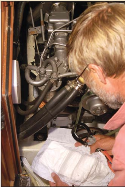
Follow the procedures specified in your owner's manual to bleed the engine after changing fuel filters.
