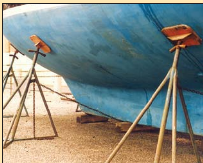
Good: Join jack stands together with chain so stands don't spread under load and collapse.
