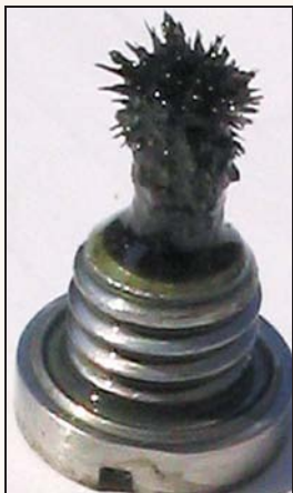
Metal filings on gearcase fill screw magnet.
