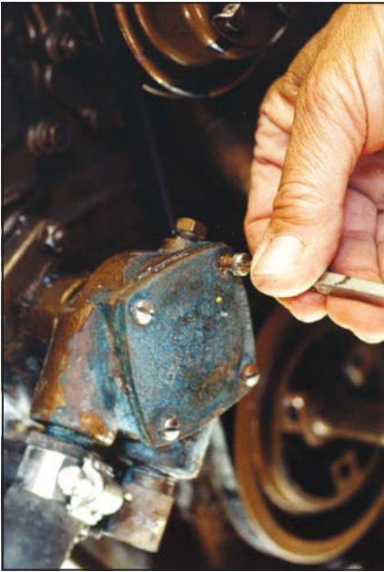
(top) Worn impeller with vanes that have taken a "set." (left) Remove the waterpump impeller to access the impeller.
