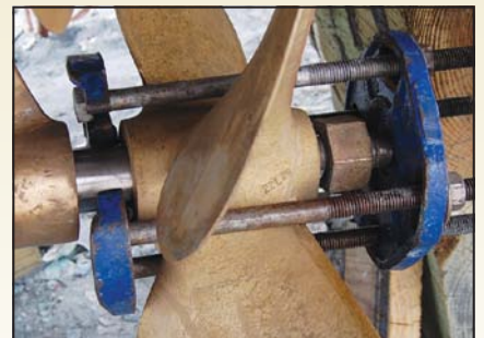
Plate puller installed on four-blade propeller. The plate with the U-shaped cutout fits behind the propeller, between the prop and the strut, the flat plate mounts on the shaft end and threaded rods run between the blades. To use, tighten the bolts on the end of the rods and the prop pulls loose.
