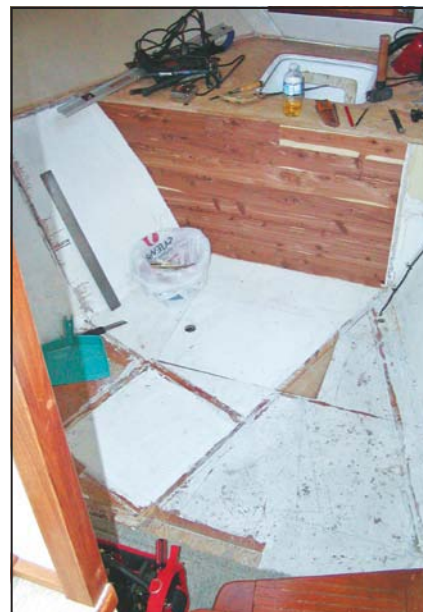
Demolition of the vee berth complete.
