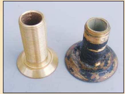
Note the difference in size between the flange on the old thru-hull fitting and the new one. Luckily, the old one was in perfect shape and could be reused.
