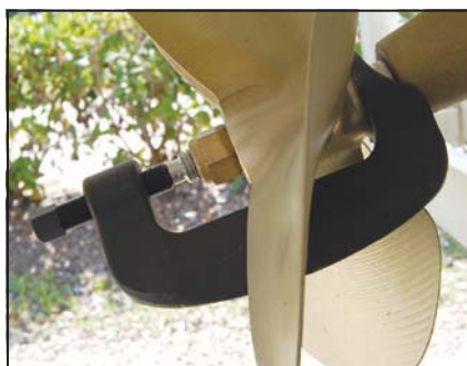
C-clamp style puller installed on inboard engine ski boat. Tighten the bolt on the end of the clamp and off comes the prop. This device fits three- and four-blade ski boat-type propellers and other small props on 1" (25mm) and 1-1/8" (28mm) shafts.
