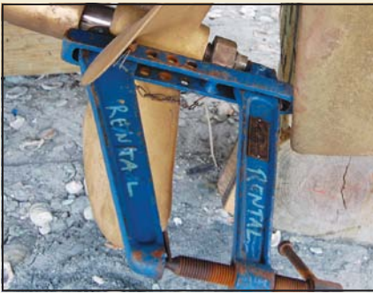
Scissors-type puller at work. Crank the outside handle and the inner jaws squeeze together and loosen the propeller.
