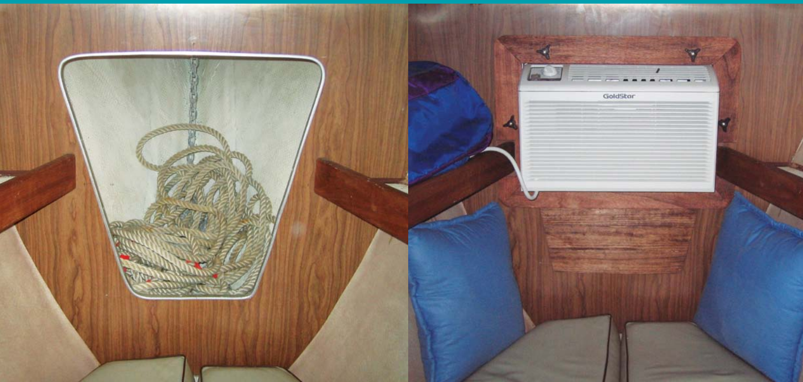
(left) Before: Original forepeak with anchor line storage. (right) After: Modified forepeak now holds a household air conditioner that is easily removed for storage off the boat or for quick access to the forepeak, if needed.
