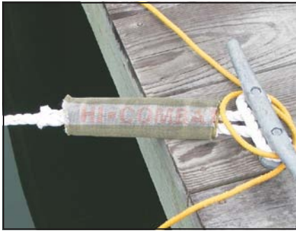
Heavy-duty hose prevents line from chafing against dock edge.
