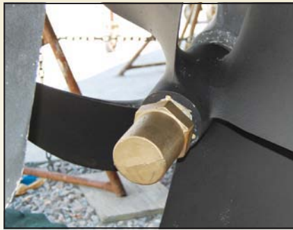
Prop knocker installed on four-blade propeller with 2-1/4" (57mm) shaft, tightened against the end of the shaft. A few good whacks and off comes the prop.
