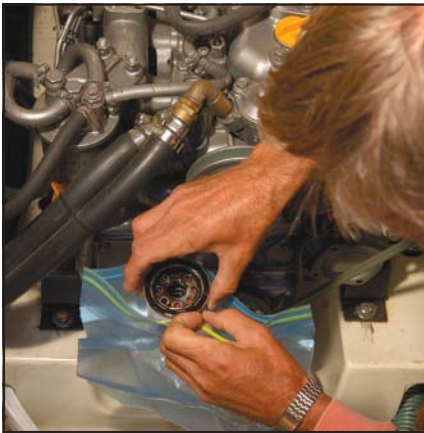
(top) Two necessary oil change tools are a strap wrench to loosen the oil filter and a diaper or other absorbent material to catch any spills. (bottom) Place used fuel filters in a closable plastic bag for disposal at a hazardous waste collection facility.
