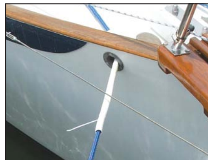
A section of white hose secured with cable ties covers the bow line as it passes through the chock.
