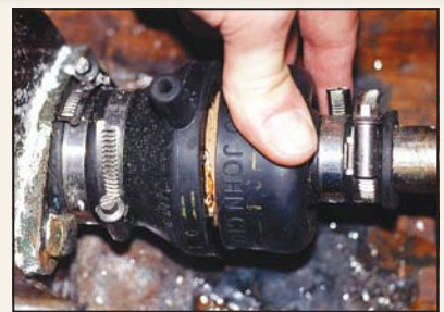
Some mechanical shaft seals require a "burp" after launching.
