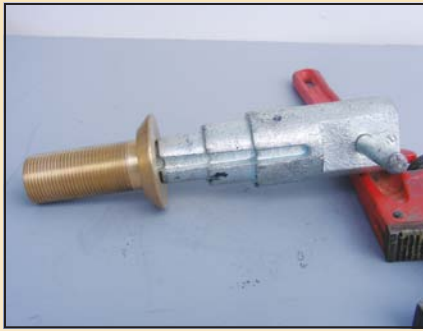
Thru-hull tool the author used to remove the old thru-hull,
