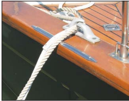
(top) A fabric sleeve protects the line and a metal rub strake prevents damage from the chain. (bottom) Stainless-steel rub strake provides a smooth surface for line to cross and, at the same time, it protects the varnished surface of the toerail.
