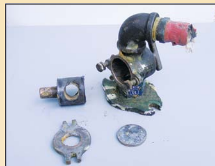
The failed 30-year-old Groco rubber plug seacock.
