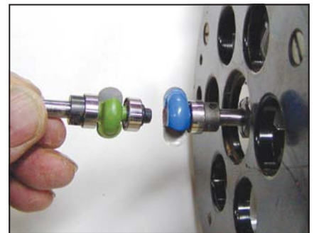
Shown in green is the original router bit. The modified one that the author purchased for $15 is blue.
