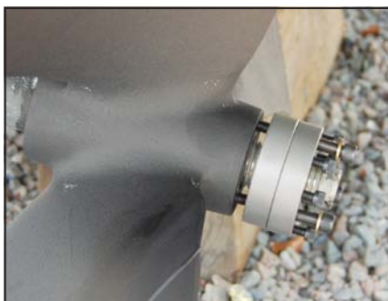
Prop Smith threaded on the end of the shaft. Bolts thread into holes in the propeller. When tightened, the bolts pull off the prop. The split plate design also allows reinstalling the prop by tightening the smaller bolts, pushing the forward plate toward the prop so it slides up the shaft taper until it seats.
