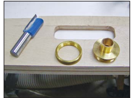
Simple jig made to cut the drawer pulls.
