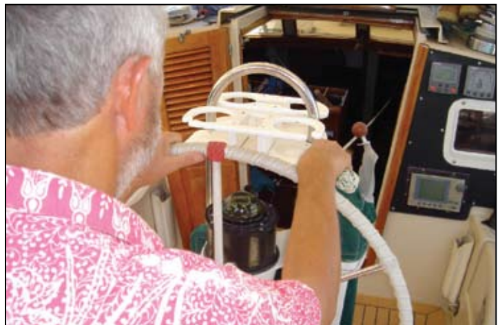
The author operates the anchor flaker, a simple rope-powered device that with a little practice lays chain as well as any human could.
