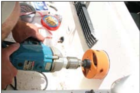
Before cutting your boat, make sure there is nothing behind the hole you are planning.
