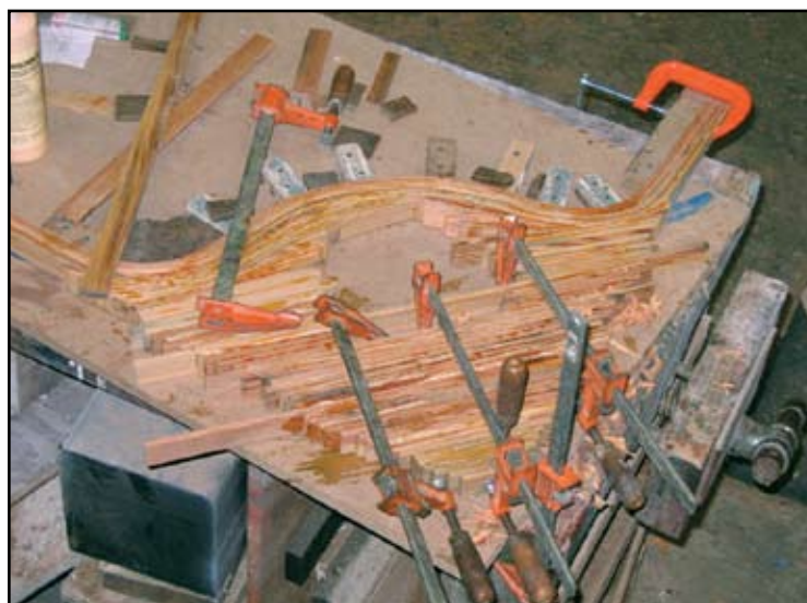
The pine strips were ripped very thin, glued and clamped three at a time to prevent breaking.
