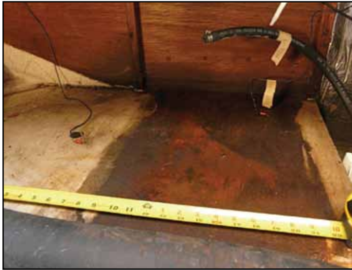
The empty location, with hoses and the sender ground wire labeled. There's room for a slightly larger tank beyond the "diesel-stain" footprint of the old tank.
