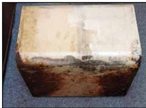
Only after removal was the author able to see the extent of the rust damage to his fuel tank.
