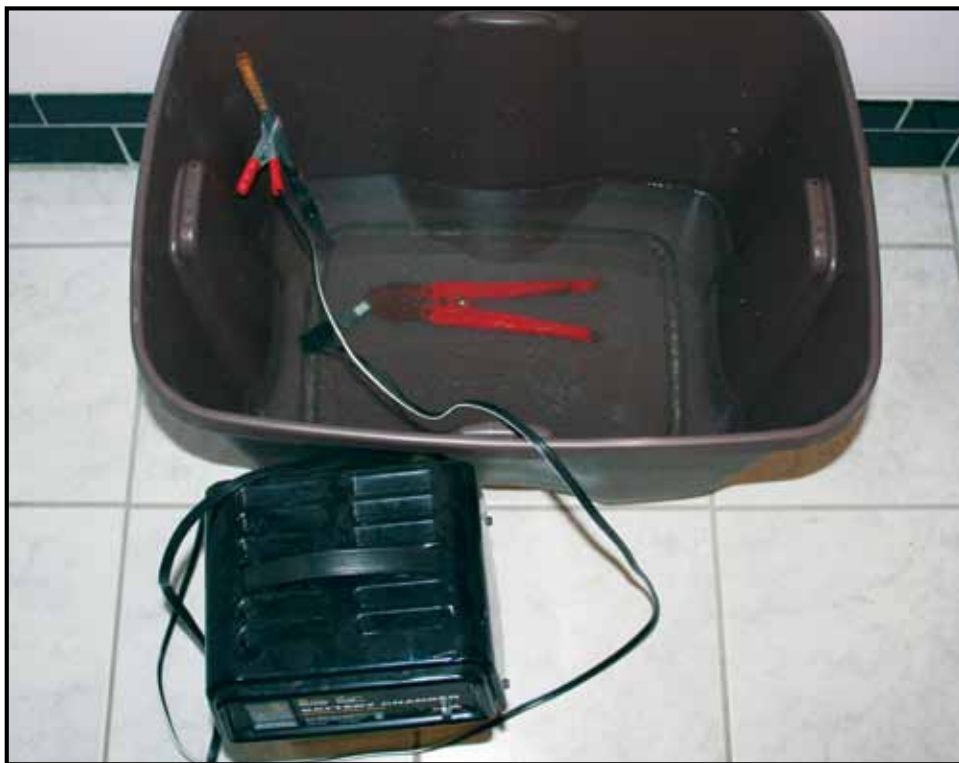
A basic electrolysis bath can remove rust in as little as 24 hours.
