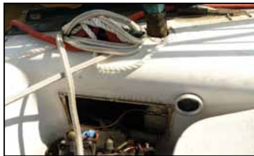
The empty location, with hoses and the sender ground wire labeled. There's room for a slightly larger tank beyond the "diesel-stain" footprint of the old tank.
