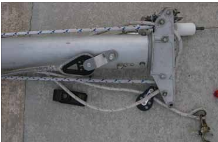
The mizzen upper shroud, attached to new clevis brackets at the masthead.
