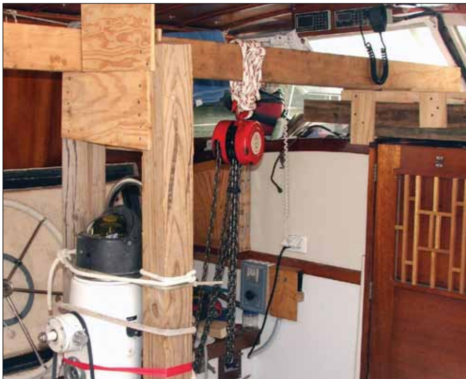
To make a solid support for the chain hoist, the author used 4-by-4 uprights and a 4-by-6 cross beam.
