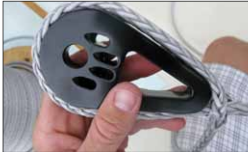
Pre-fitting an aluminum "terminator" thimble.
