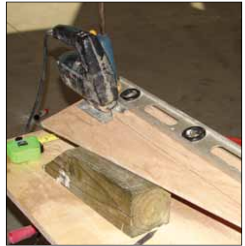
To make reassembly of the reconfigured helm easy, each of the instruments was labeled before disassembly, left. When making straight cuts, top, it's best to use a straight edge.
