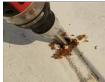
Dark, wet core spewed out of some of the holes, left. Other holes had light-colored, dry and healthy core.
