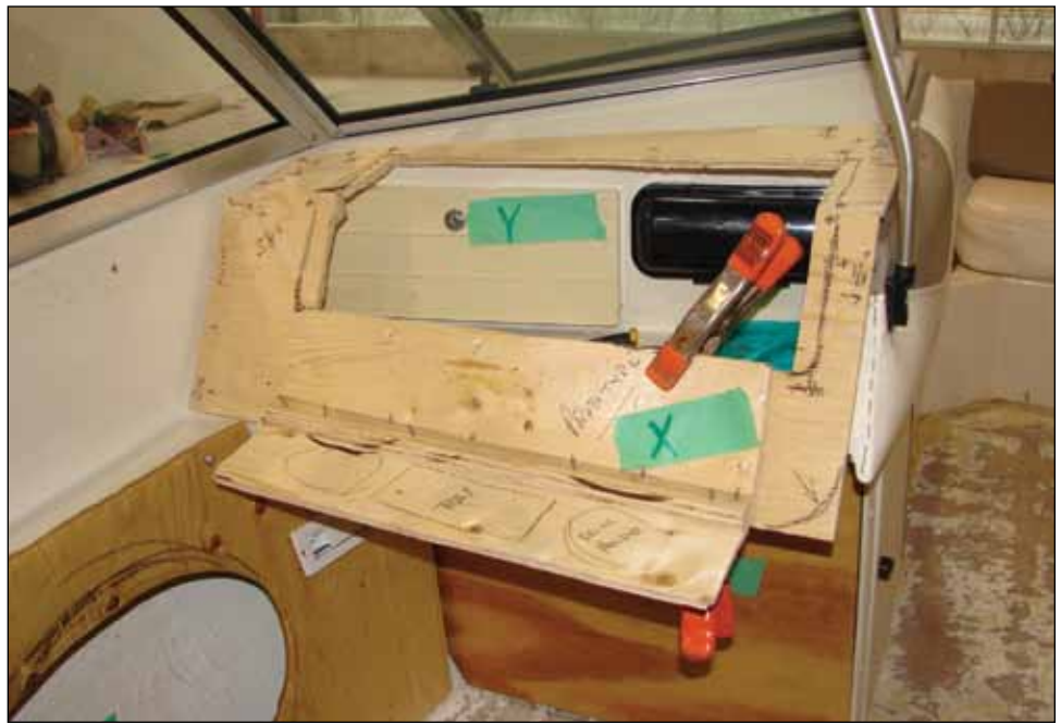
To reconfigure the dash on the passenger side to make it more accessible, scrap wood was used to create a template before any final cuts were made. Clamps kept it in place.
