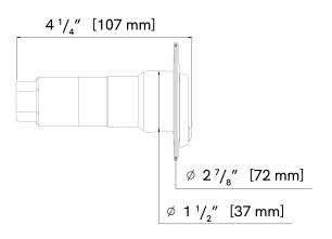
Flush-mounted stainless steel hydrant with hose connector. A reliable, leak-proof water outlet that can be used anywhere water access is needed, on land or sea. Ideal for any marine vessel or washdown application. Can be mounted horizontally or vertically. Polished stainless steel faceplate with "WASHDOWN" marking embossed and painted.
