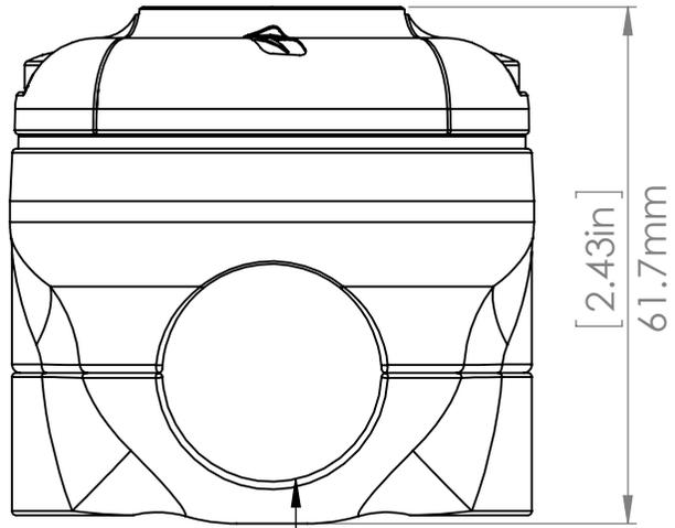
Fits 25mm (0.98in) rail or 19mm (0.75in) with supplied insert
